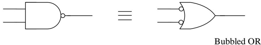
Note that OR and AND have their equivalent with two inversions (i.e. circles at input and output) while NAND and NOR have only one bubble at the input side.
